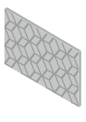
6 The interplay of washed out and smooth surfaces makes the design visible.
