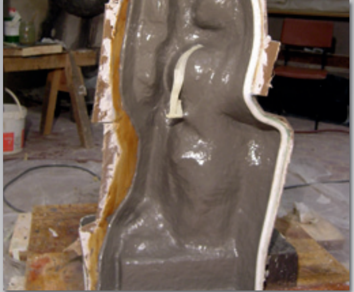
13 | Smoothed out Epoxi-GF shell
