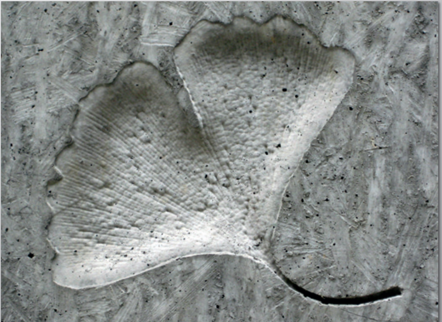
Ginkgo leaf concrete imprint modelled using PUR elastomer
