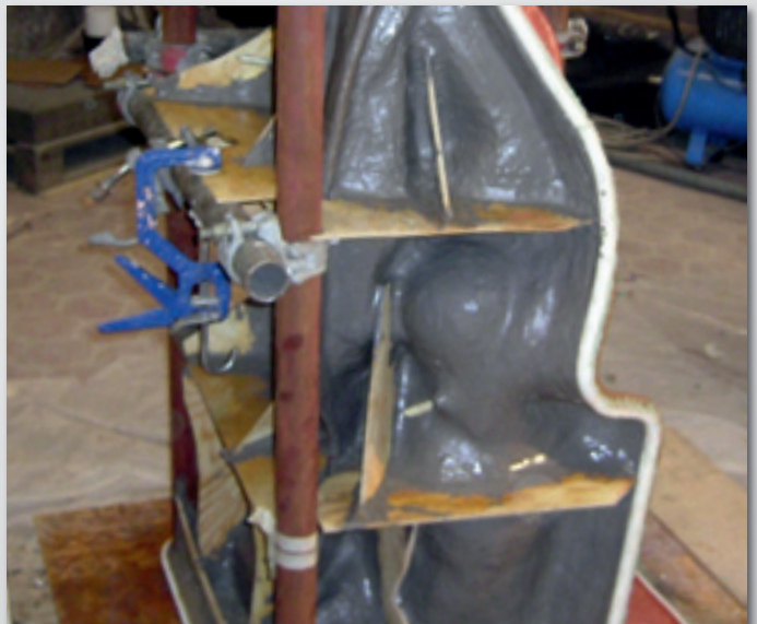
16 | Supporting and clamping of first half of mould
