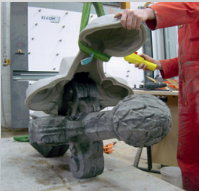
Removal of a two-piece shell mould made of PUR elastomer
