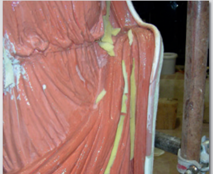
18 | Foam fillers for the back-tapering
