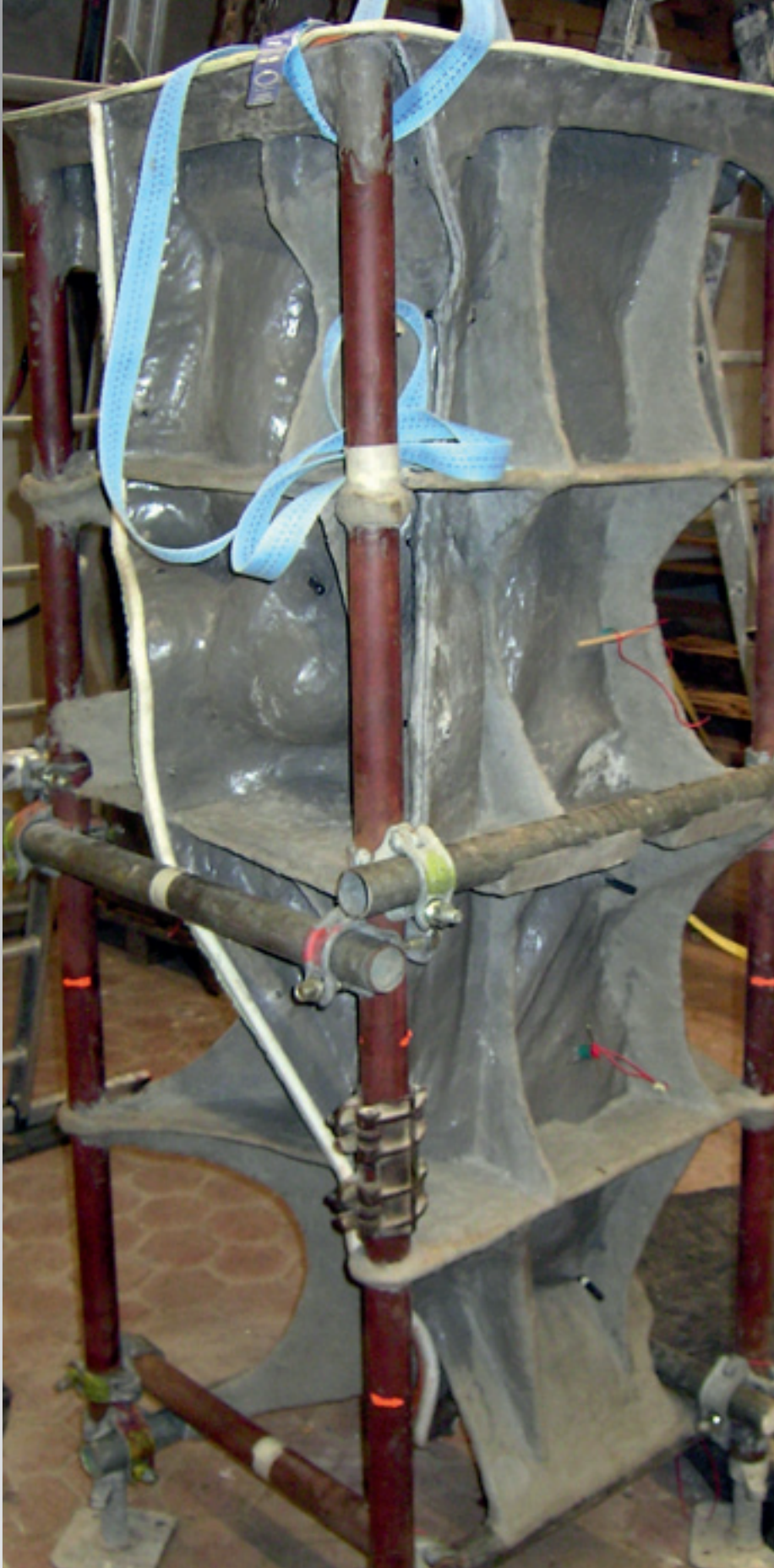
22 | Mould ready for reproduction casting
