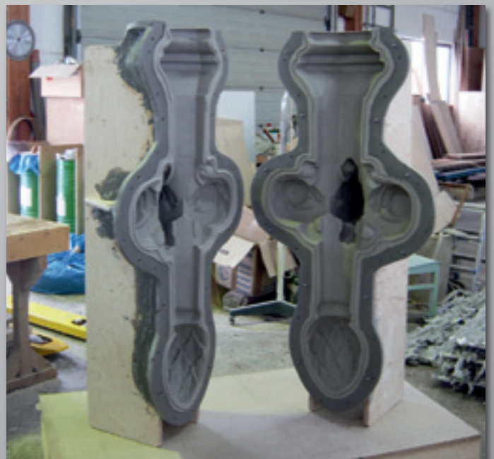
Two-piece shell mould with mould support
