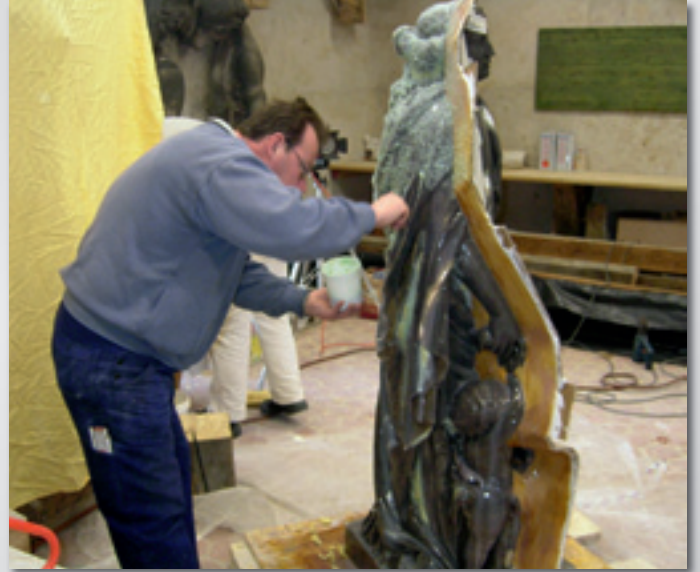
7 | Application of the second silicone layer
