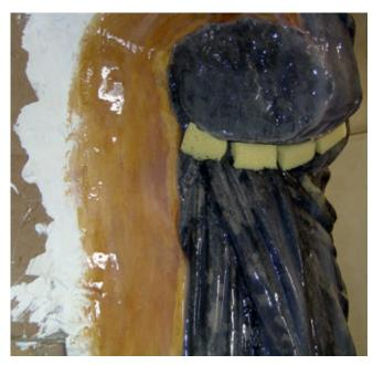
6 Placing foam fillers in back tapers or heavy dips
