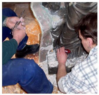
14 Removal of separation rib
