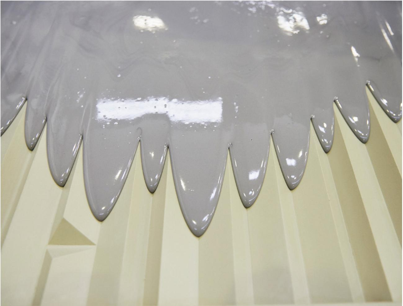
After the positive cast has been sealed with release wax, the liquid elastomer is poured onto it.
