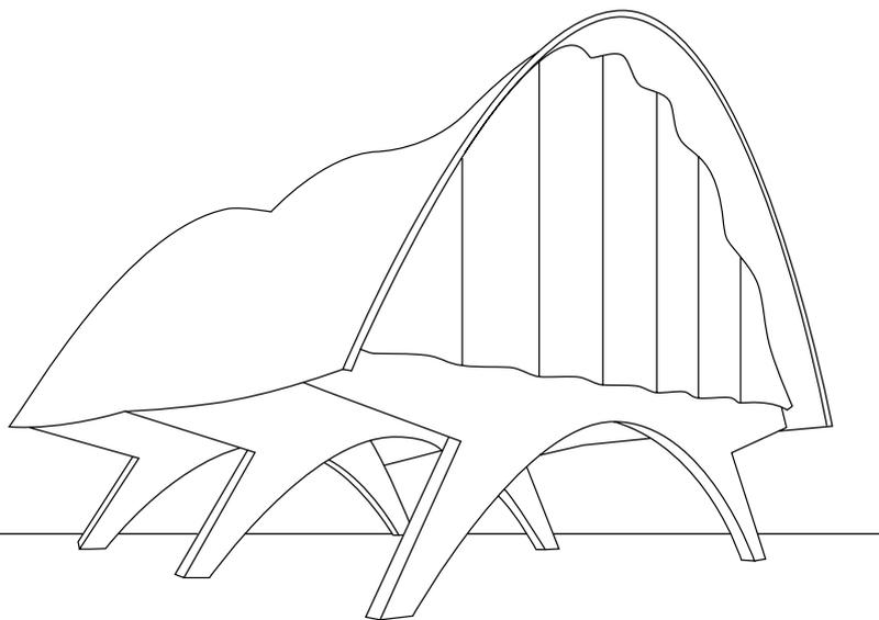
The hyperbolic paraboloid, or hypar roof held a particular fascination for Candela. It is attractive and elegant, the formwork can be manufactured from unbent wood, and its realization requires only a thin layer of concrete, which saves material and thus costs.
