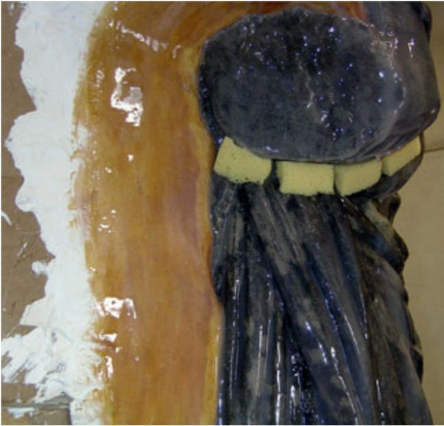
6 Placing foam fillers in back tapers or heavy dips
