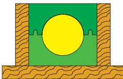
**Elastomer cast of the second half of the mould**
