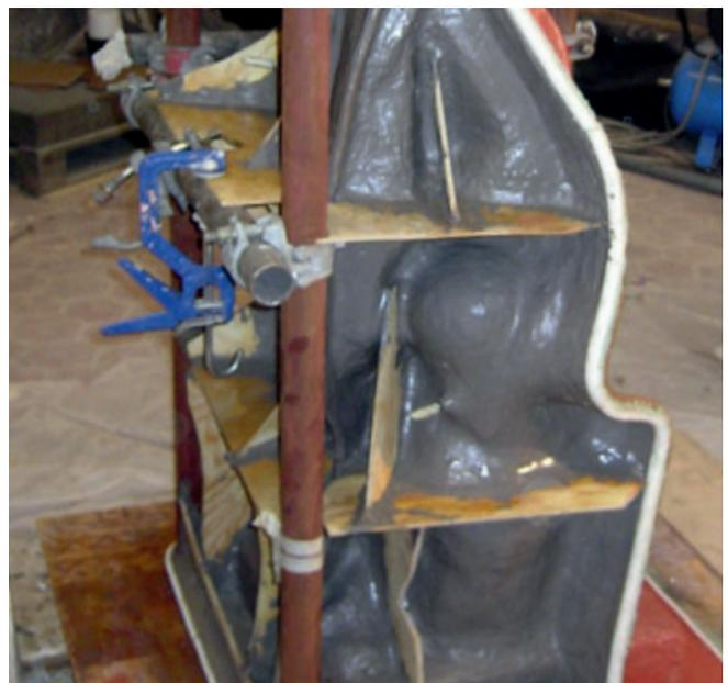
16 Supporting and clamping of first half of mould
