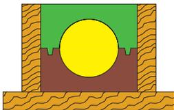
**Elastomer cast of the first half of the mould**
