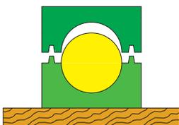
**Removing the two-part mould**
