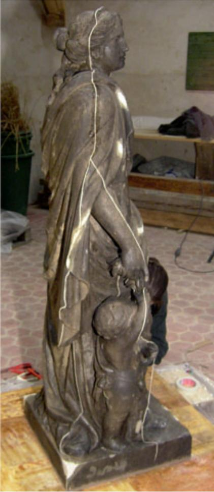
1 Determining the parting lines
